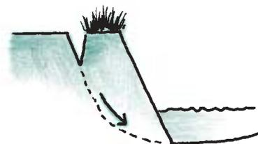
d. Slumping failure (slope failure → toe failure → base failure)
