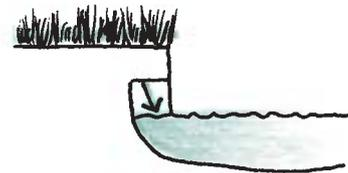
c. Slumping failure (slide → topple)
