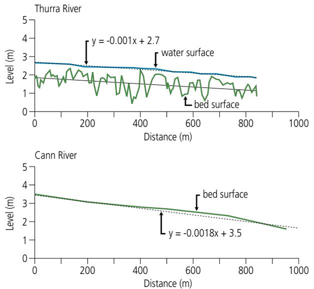
**Figure 2:** Bed profiles of the Thurra and Cann Rivers showing the profound homogenisation that occurred following wood removal and subsequent channel erosion (the Cann River would have been similar to the present day Thurra long profile [Figure 3] prior to desnagging and riparian vegetation disturbance). (A. Brooks)
