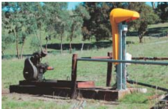
Solar powered pump with back up petrol pump. Solar panel shown above right. Photos Roger Charlton.
