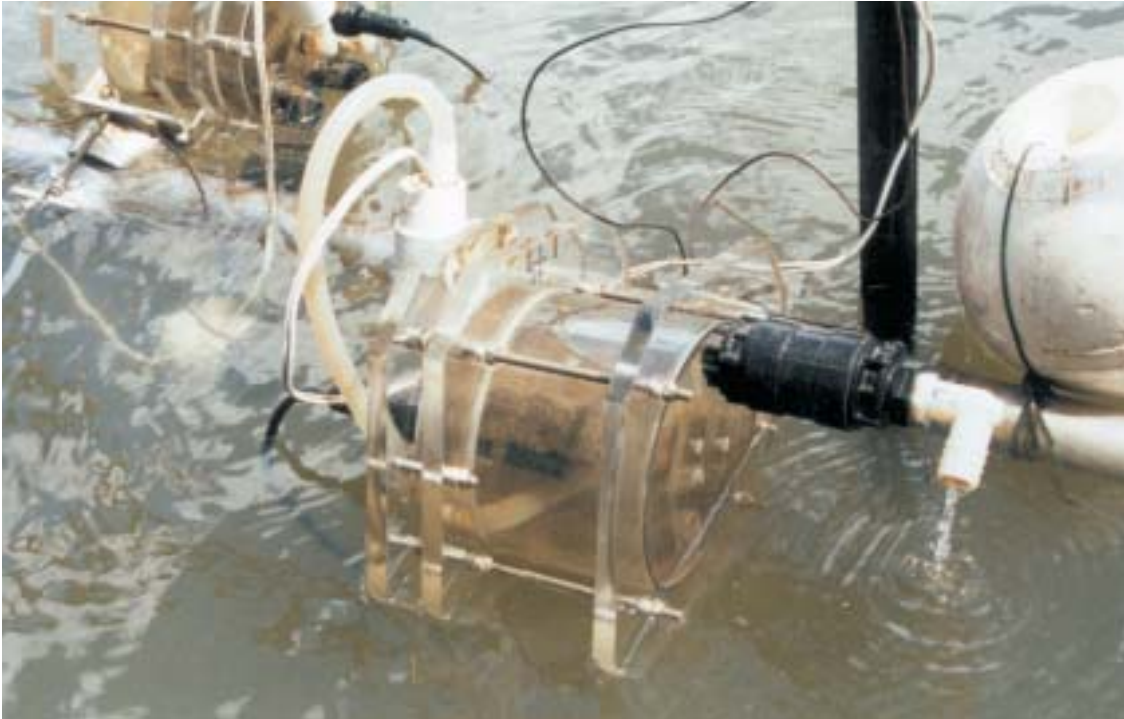
Chambers used to measure the production and consumption of nutrients and energy in riverine systems.
