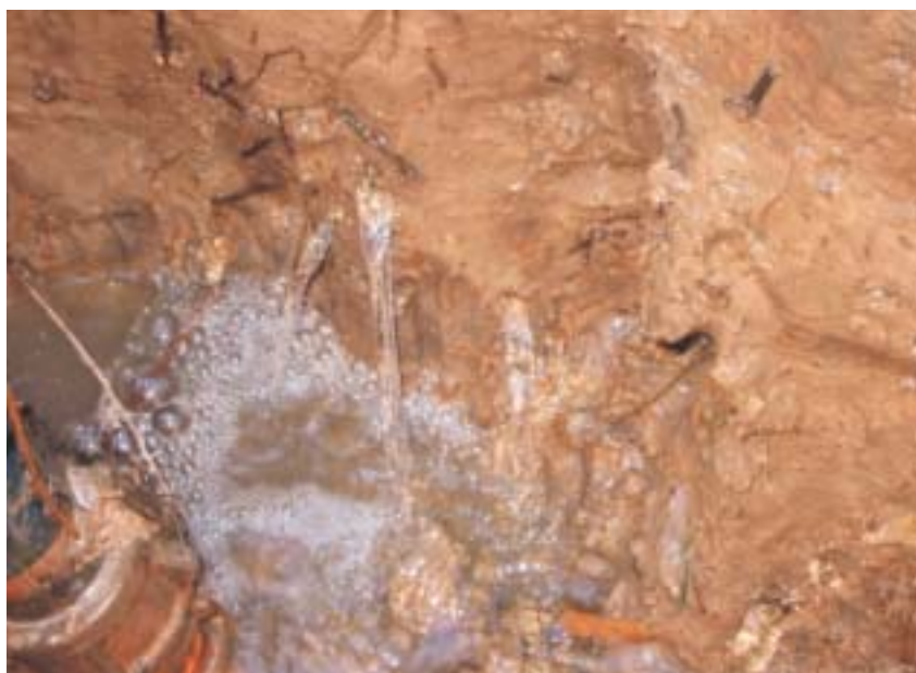
Figure 2: Acid groundwater flowing through soil macropores rapidly filling an excavated pit. Even though this acid sulfate soil has a clay texture, it has high hydraulic conductivity and rapid lateral movement of groundwater due to the network of interconnected pores and cracks. Photo Thor Aaso.
