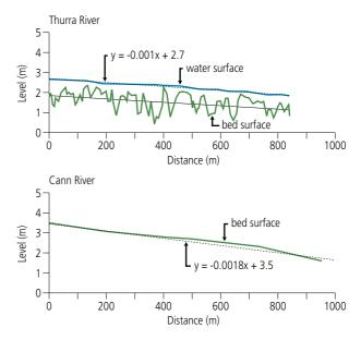
**Figure 2**: Bed profiles of the Thurra and Cann Rivers showing the profound homogenisation that occurred following wood removal and subsequent channel erosion (the Cann River would have been similar to the present day Thurra long profile [Figure 3] prior to desnagging and riparian vegetation disturbance). (A. Brooks)
