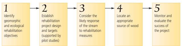
Key steps associated with the design and evaluation of wood reinstatement. Although presented as a linear process here, planning for the reintroduction of wood should be an iterative process.
