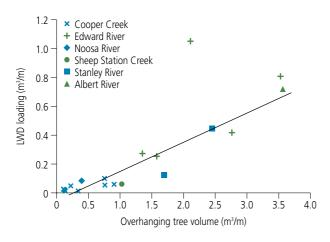
**Figure 4**: Stream wood loading and fringing riparian overhanging tree volume along six south-eastern Australian streams (from Marsh et al. 2001).
