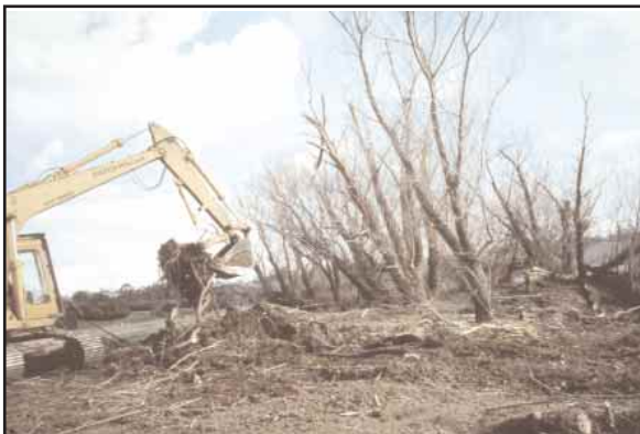
Figure 75. Gripping arm or ‘thumb’ attached to bucket used for willow removal on the La Trobe River, Victoria.
